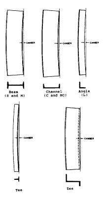
Positions for Measuring Camber of Shapes
