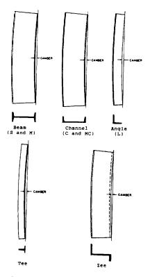
Positions for Measuring Camber of Shapes
